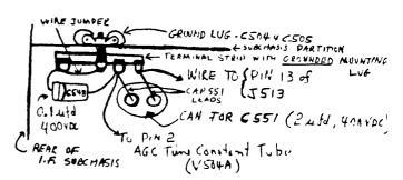
sions onto the cap leads, and these were taped to the body of the cap with good plastic tape. In making this repair, I also replaced C548 with a new 400-VDC Mylar-type unit. It is physically in the way and is rated at 100 VDC. In order to insure good mechanical rigidity, it seemed wise to mount a terminal strip on the chassis partition where C504 and C505 are gounded. A diagram is above.
