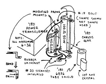
mounted a terminal lug underneath. The high wattage was necessary to get the resistors to run reasonably cool (about  $55^{\circ}$  C). A sketch of the mounting arrangement is above.
